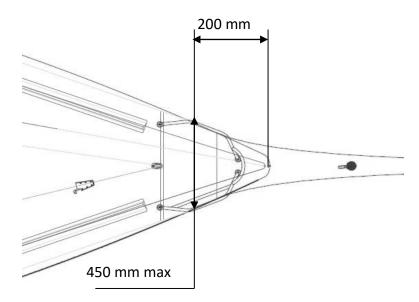
The cockpit can be any width between the aft-most point used to determine  $\underline{Lh}$  and 1.75 metres forwards of this point.
